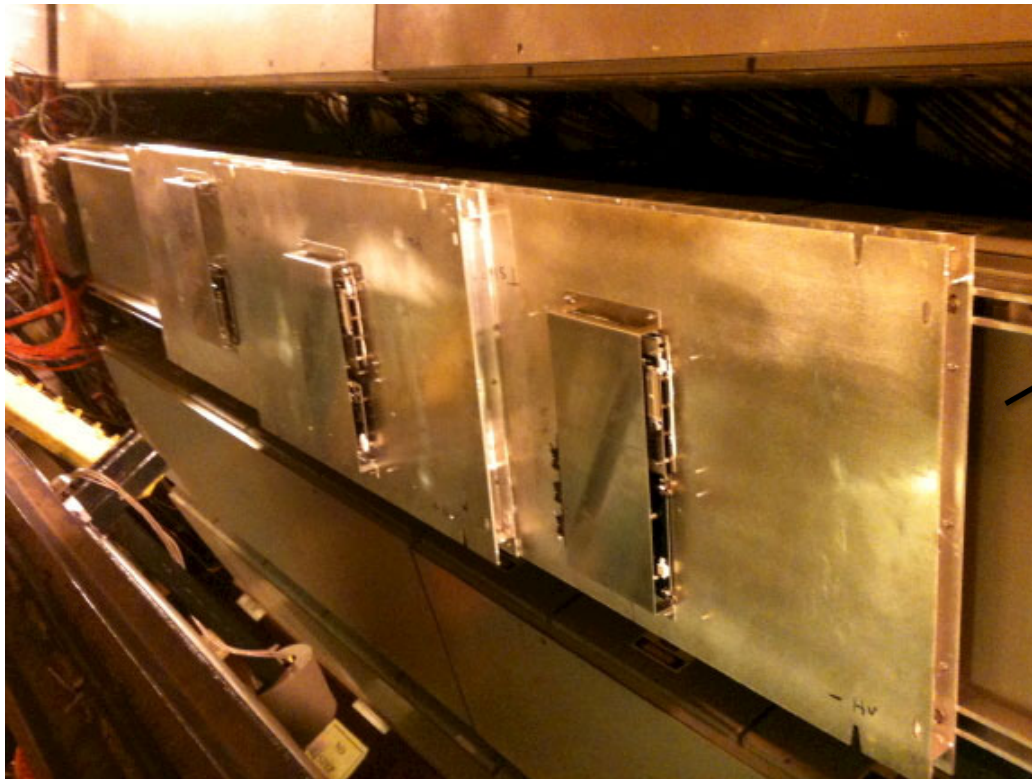
Three MTD11 trays (craned into place)
