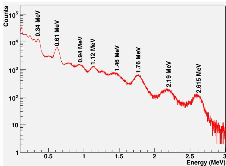
Figure 6: The spectrum from a stone sample following the MCA bin to energy calibration and including the expected positions of the peaks from specific naturally occurring radionuclides.
