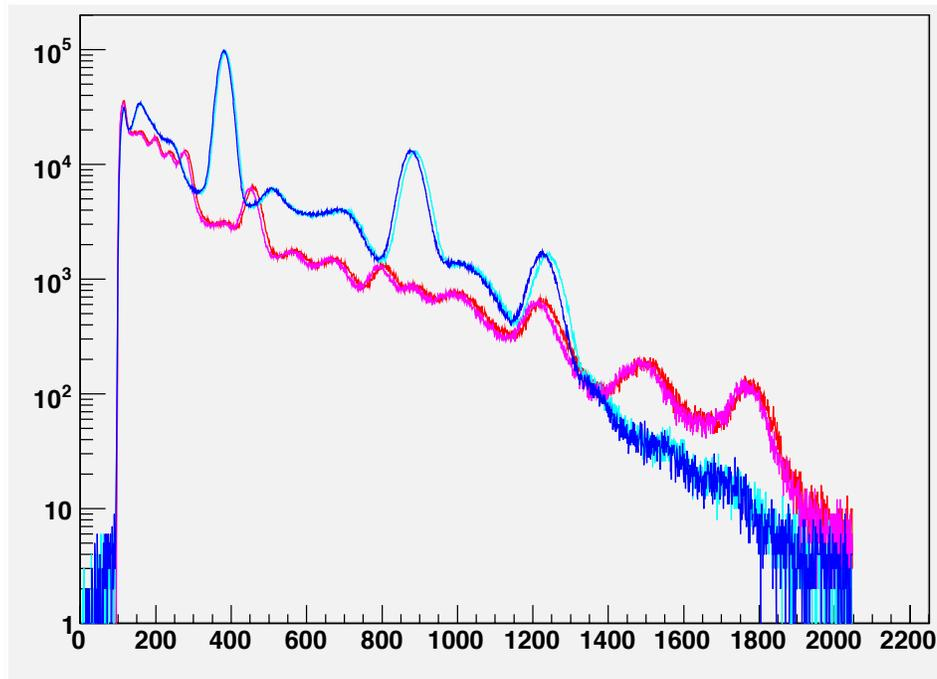
Figure 1: *The raw spectra from two runs with a  $^{22}\text{Na}$  source (blue and cyan) and from a section of a granite countertop (red and magenta). The vertical axis is counts, and the horizontal axis is the MCA bin number.*
