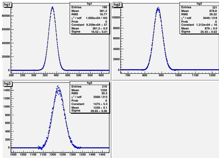
Figure 3: The three peaks from the  $^{22}\text{Na}$  source following the subtraction of the background around each peak using the exponential fits shown in Figure 2. The vertical axis is counts, and the horizontal axis is the MCA bin number.
