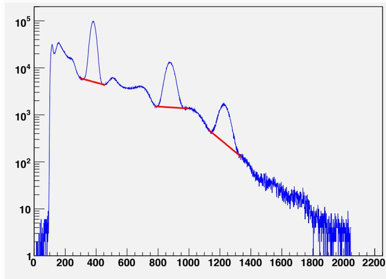
Figure 2: A raw spectrum the  $^{22}\text{Na}$  source. The vertical axis is counts, and the horizontal axis is the MCA bin number. The red lines are exponential fits to the “background” around each of the three peaks.
