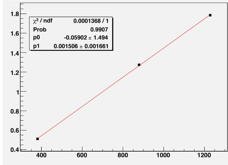
Figure 4: *The MCA bin number to energy calibration. The vertical axis is energy in MeV, and the horizontal axis is the MCA bin number.*
