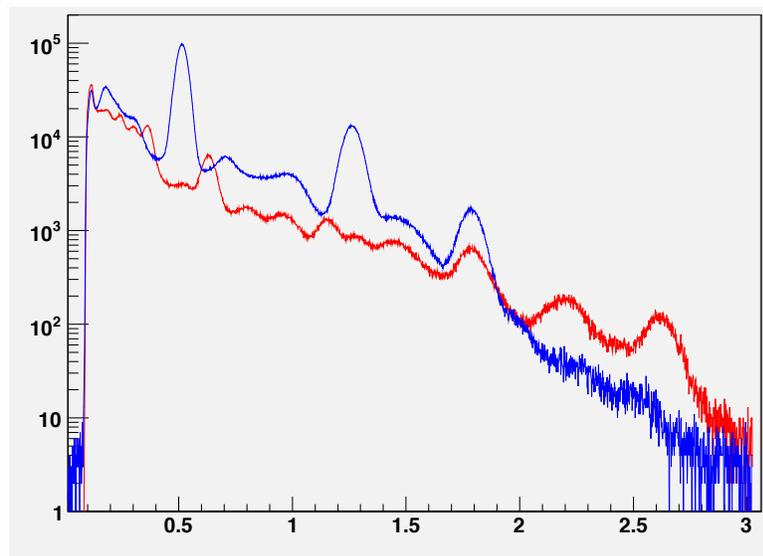
Figure 5: The gamma spectrum from the <sup>22</sup>Na source (blue) and a stone sample (red) following the MCA bin to energy calibration. The vertical axis is counts, and the horizontal axis is the energy in MeV.
