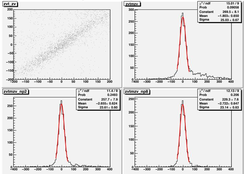
$\sigma \sim 20-25$ cm is consistent with a single detector time resn of ~1ns which is the expected value in absence of a slewing/offset correction (not enough events)
