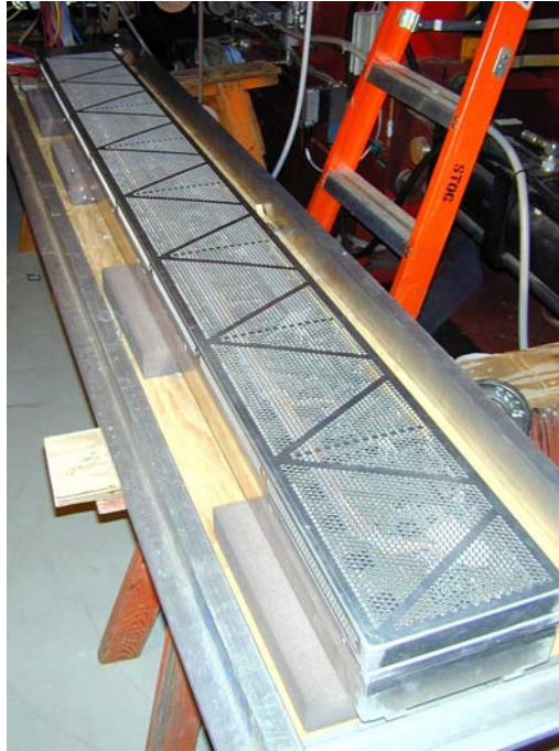
Figure 10: The TOFr5 tray with the outer perforated cover installed, shown just before the tray was installed in STAR for Run-5.
