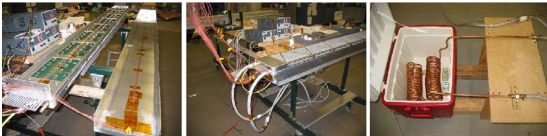
Figure 19: Shown on the left is the TOFr5 bottom and top assemblies and the thermocouple wiring for the interior of the gas box. In the center, TOFr5 reassembled and running during these tests, and on the right is the heat exchanger.
