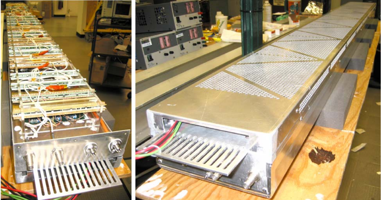
Figure 4: On the left is the interior of the TOFr5 system with 32 MRPC detectors installed, and on the right is the TOFr5 system closed up and ready for installation in STAR.
