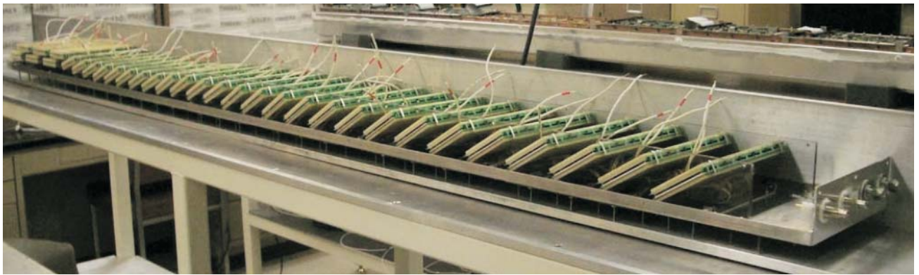
Figure 1.2: TOF tray without top cover, notice the 32 MRPC modules.
