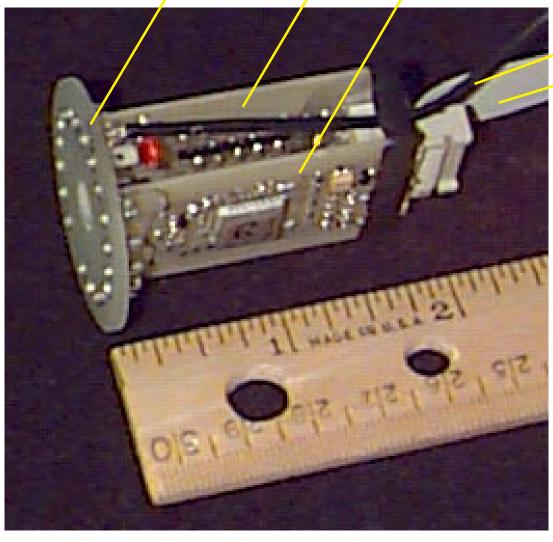
PMT Anode signal, RG-174 HVSys Bus
