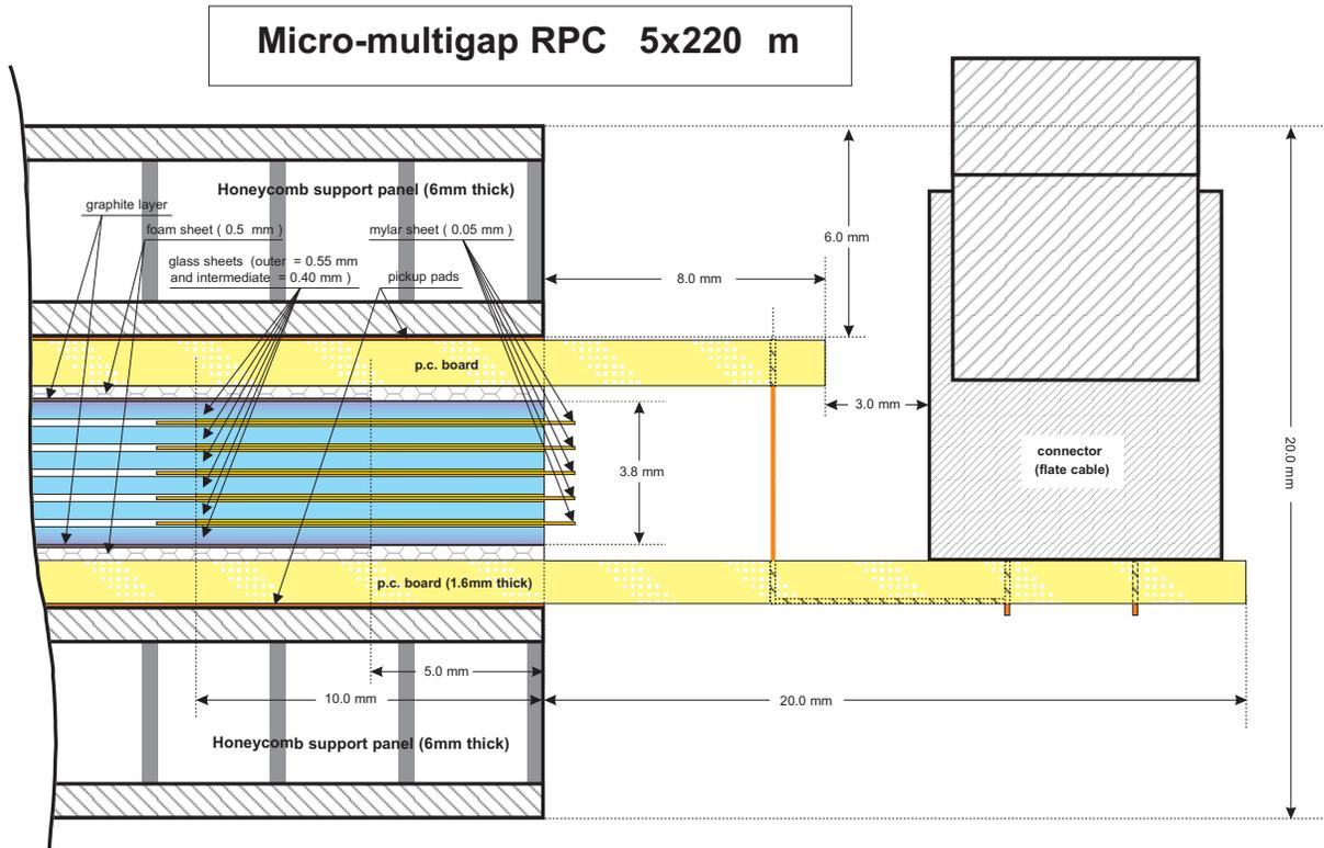
Fig. 1. A partial sectional view of a multi-gap RPC TOF module.
