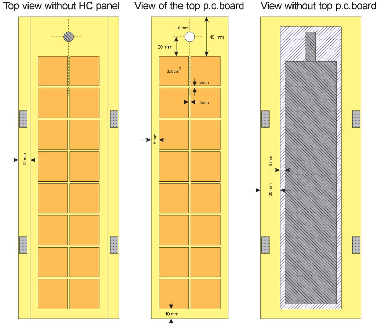
Fig. 2. The first two images show the p.c. boards with the copper pads. The third image shows the glass cell (light shading) sitting on the bottom p.c. board with the graphite H.V. electrode (darkest shading) shown on top of the top glass layer.
