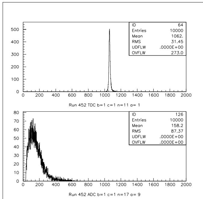
Fig. 4. (top) The raw TDC distribution for Rice 4 card 1 channel 2 is shown. The overflow count represents the chamber inefficiency. (bottom) The raw ADC distribution for the same cell.
