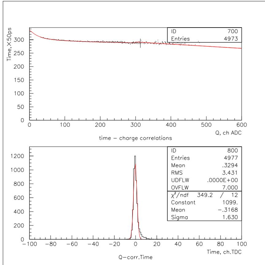
Fig. 5. (top) The time versus charge distribution for Rice 4 card 1 channel 2 is shown. This information is used to correct the raw time distribution. (bottom) The charge corrected time distribution for the same cell. The sigma is 1.63 or 81.5 ps.
