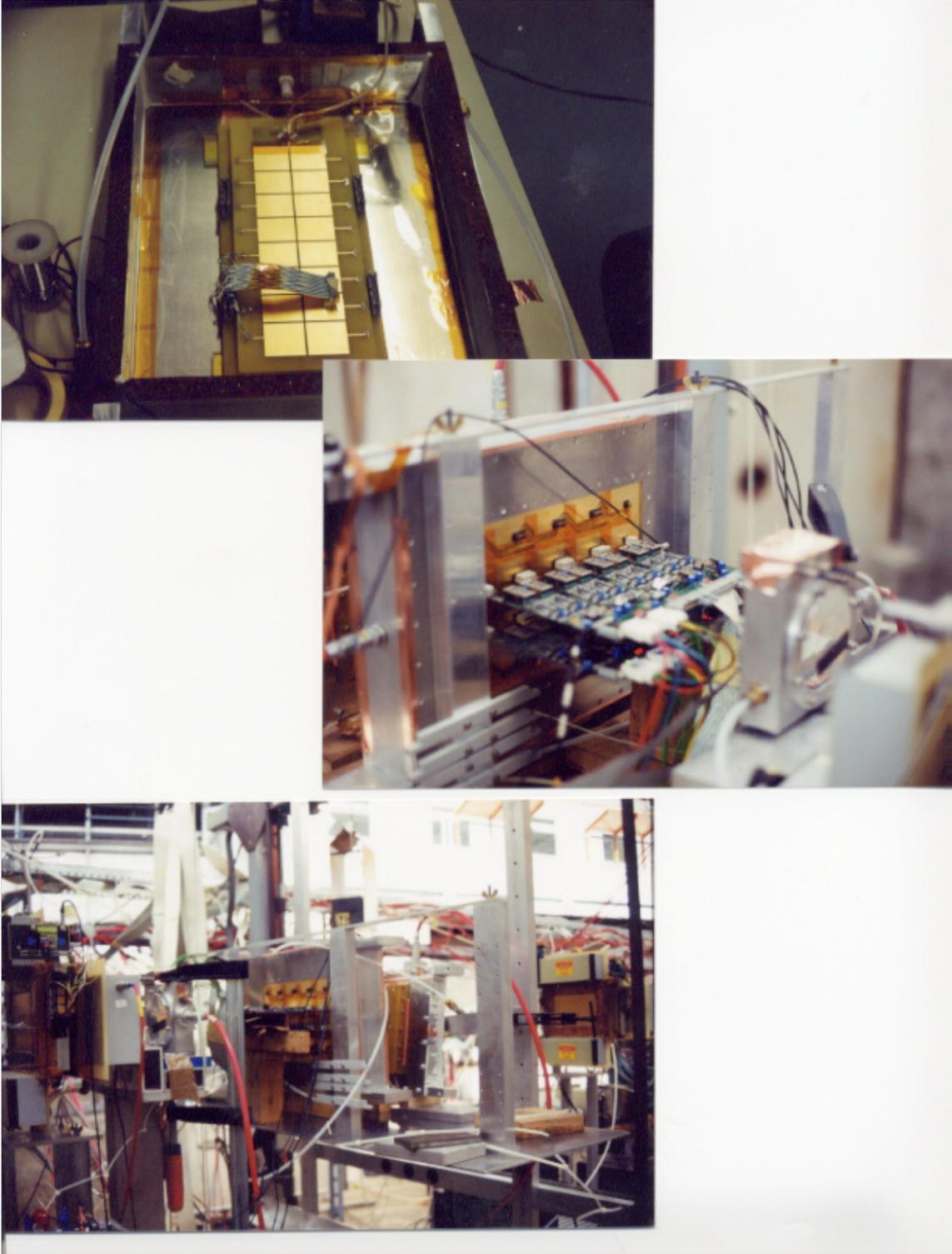
*Fig. 3. The top picture is the test RPC TOF module RICE 4 in a gas Box. The middle picture shows the test module in the beam line with front end cards installed. The lower picture shows more of the beam line. The two of the start detectors, crossed strips of scintillator are visible to the right.*
