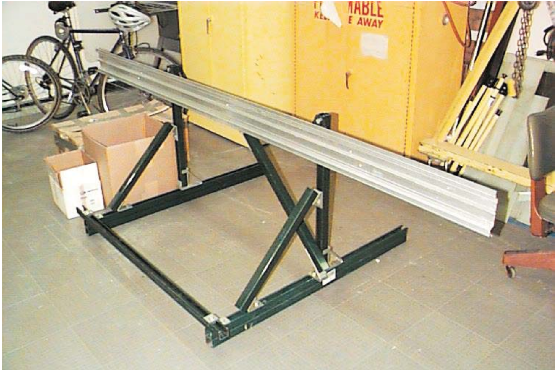
Stand to hold tray in test-beam setup
