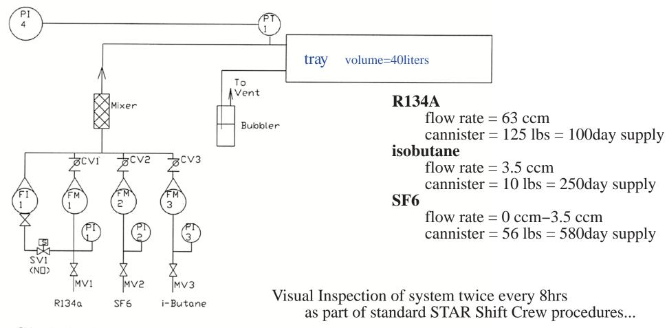
CV- check valve MV-manual valve FI-flow indicator FM-mass flowmeter PI-pressure indicator SV-solenoid valve PT-pressure transmitter
