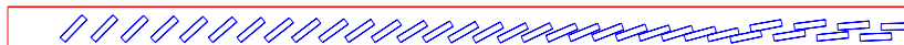
Fig. 2. The profile view of 34 RPC TOF 6-channel modules in a CTB tray.
