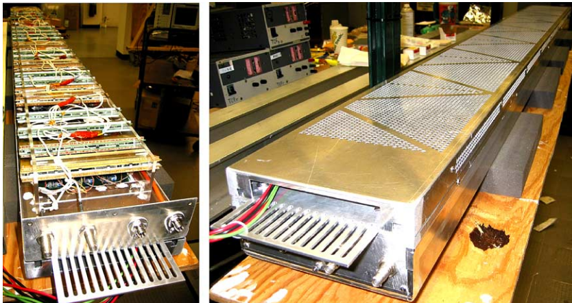
Fig. 4. On the left is the interior of the TOFr5 system with 32 MRPC detectors installed, and on the right is the TOFr5 system closed up and ready for installation in STAR.
