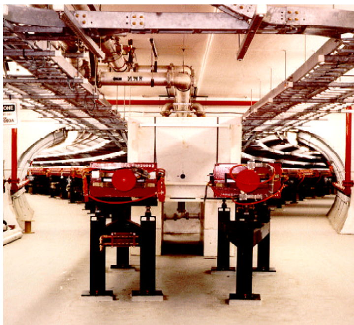
ATR Initial Beam Test brings ions to this point. Later, the ATR switching magnet will send ions into either the X line (left) and blue (clockwise) ring or the Y line (right) and yellow (counter-clockwise) ring.
