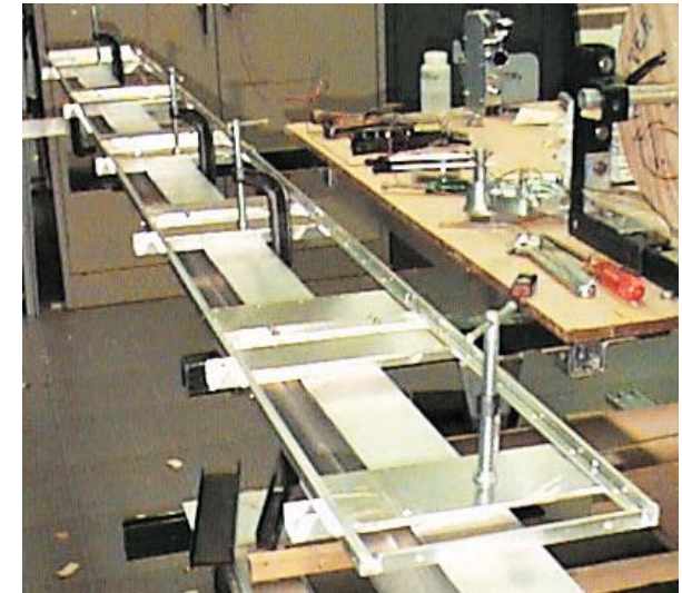
welded/tapped rail assembly (glued gaskets also)
