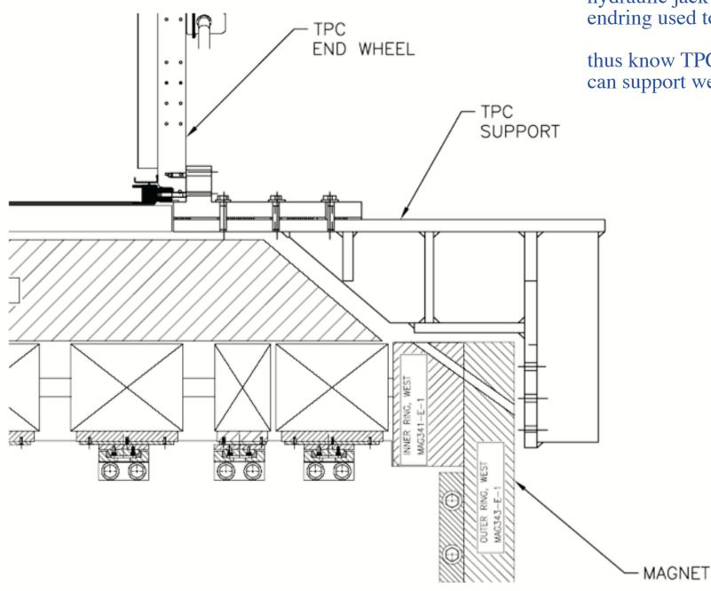
During BEMC installation, hydraulic jack on TPC support endring used to support TPC.
