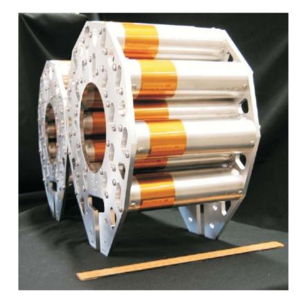
Primary Function provide start-time needed to form  $1/\beta$  from the stop-side data calibrates independently from stop-side calibration does not require any information other than that from the upVPD itself
