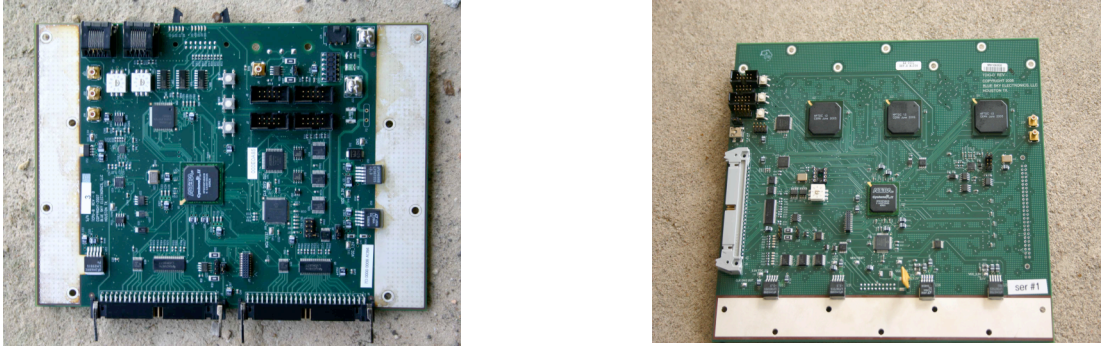
Figure 4: TCPU data readout card (left) and TDIG TDC card (right)
