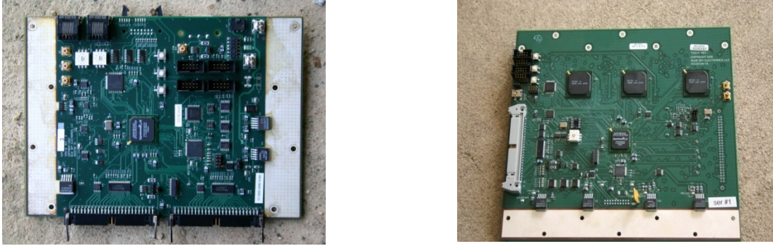
Figure 4: TCPU data readout card (left) and TDIG (PicoTOF 25) TDC card (right)
